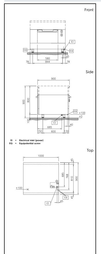
**Electric** Supply voltage: 400 V/3N ph/50/60 Hz Total Watts: 5 kW **Key Information:** Oven working Temperature: 60 °C MIN; 300 °C MAX Oven Cavity Dimensions (width): 575 mm **Oven Cavity Dimensions** (height): 300 mm Oven Cavity Dimensions 700 mm (depth): External dimensions, Width: 1000 mm External dimensions, Depth: 900 mm External dimensions, Height: 550 mm Net weight: 107 kg Configuration: One-Side Operated Oven GN: GN 2/1
